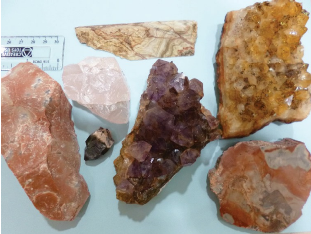
Figure 2.3 | Examples of the different varieties of quartz (jasper, rose quartz, smoky quartz, agate, amethyst, citrine, and petrified wood), demonstrating the difficulty of identifying this mineral.
