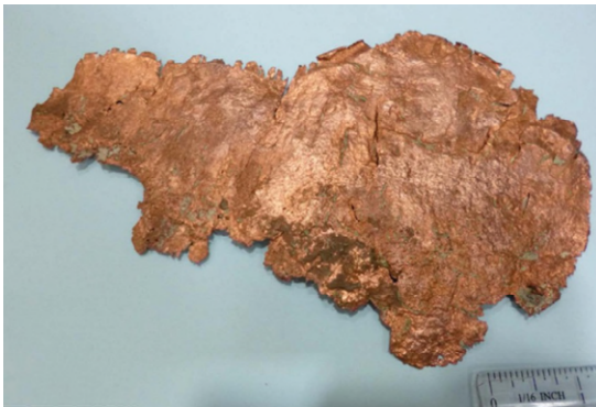
Figure 2.16 | Copper, which can be hammered into thin sheets, is malleable. Source: Randa Harris (2015) CC BY-SA 3.0
