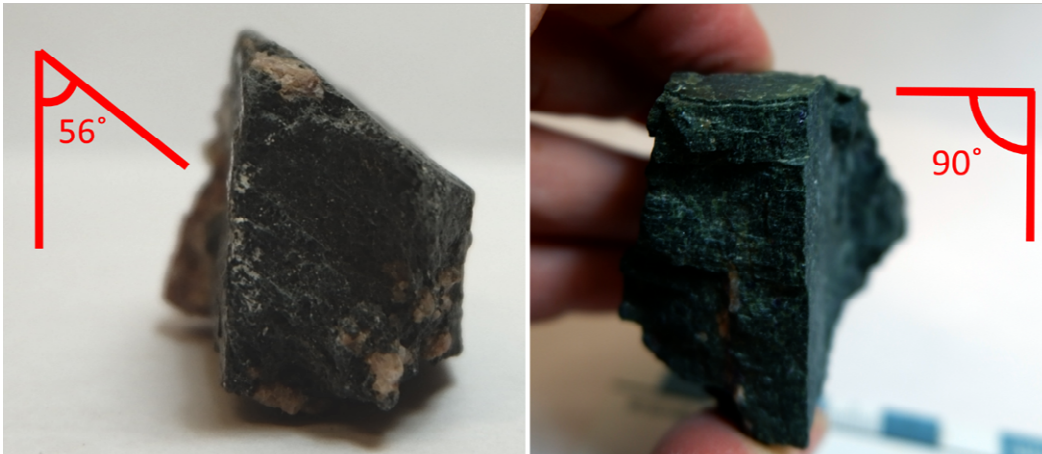
Figure 2.10 | Comparison of cleavage angles between amphibole and pyroxene. Amphibole has cleavage angles at or near 60^\circ and 120^\circ , and pyroxene has angle at or near 90^\circ . Source: Joyce M. McBeth (2018) CC BY 4.0, after Randa Harris (2015) CC BY-SA 3.0
