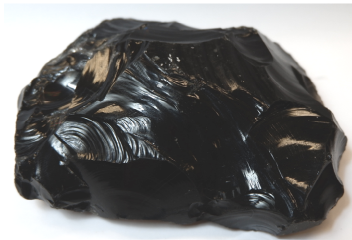
Figure 2.11 | This piece of igneous rock called obsidian has been hit with a hammer and is displaying conchoidal fracture. Source: Joyce M. McBeth (2018) CC BY 4.0
