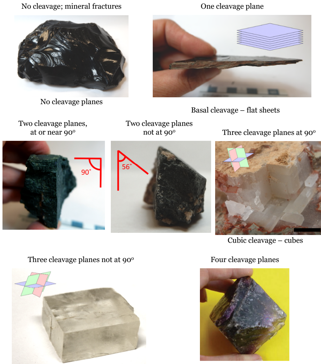
Figure 2.9 | Main types of cleavage, along with illustrations indicating the cleavage angles and directions.
