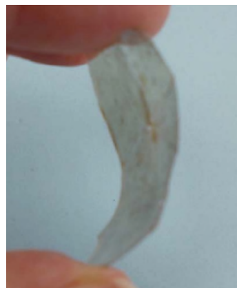
Figure 2.17 | Muscovite mica, which bends but returns to its original shape, is elastic. Source: Randa Harris (2015) CC BY-SA 3.0
